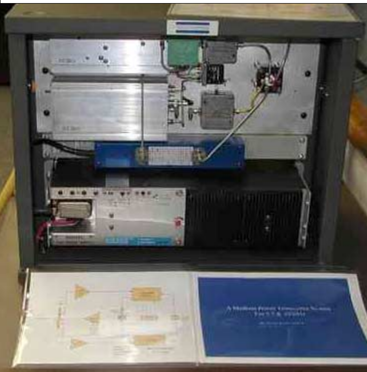
N3FTI 5 & 10G amp, showing DEMI XVTRS and LNAs, TWT, PS
